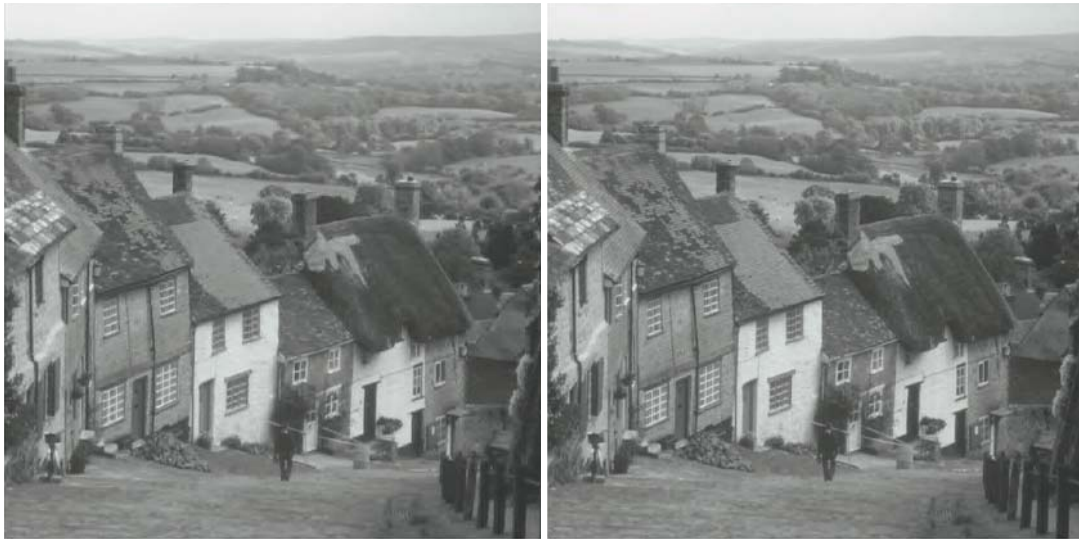
Figure 10: Left: Goldhill compressed with alchimage at 0.875bpp. Right: Original Goldhill image.
